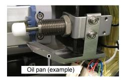
Even if an oil pan is installed, periodic replacement of shock absorbers is still required in order to prevent reduction of shock-absorption capability.
